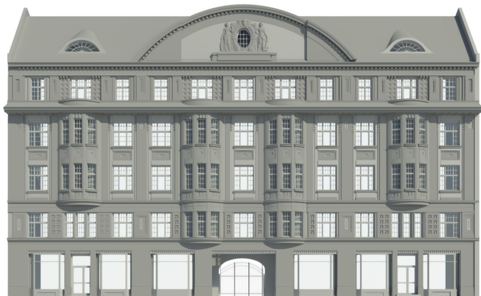
Facade 3D CAD Model from Point Cloud
