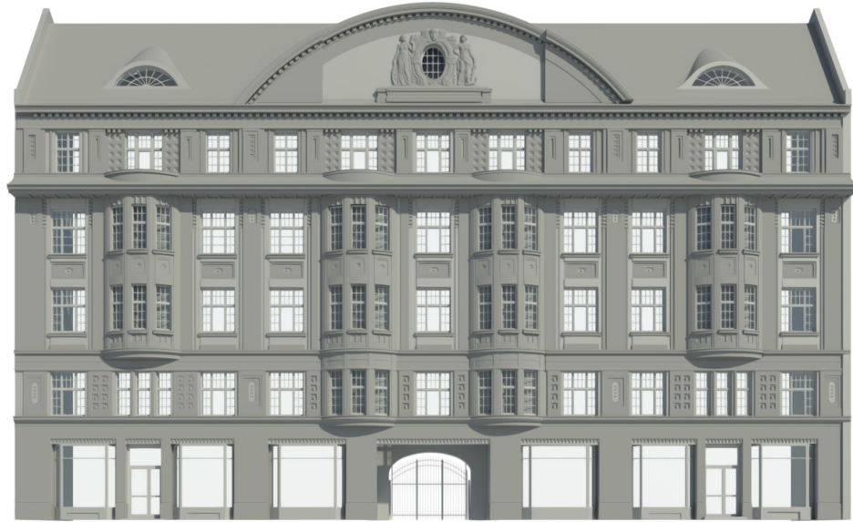
Facade 3D CAD Model from Point Cloud
